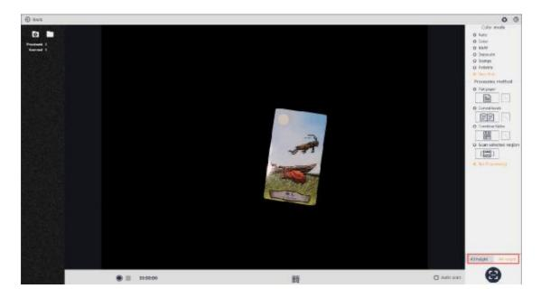
In the lower right corner of the interface, you can select the format of the preview by adjusting the height of the lifting rod of the device to set A3, A4 format (some models support the adjustment of the lifting rod). When you adjust the device for A3 or A4 format, you need to manually select the corresponding A3 or A4 format.
